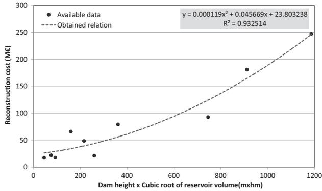
Figure 5. Relation obtained to estimate dam reconstruction cost as a function of dam height and reservoir volume.
