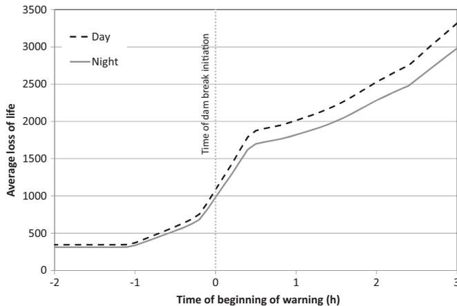
Figure 4. Relation between loss of life and time of beginning of warning to the population in the dam 4.
