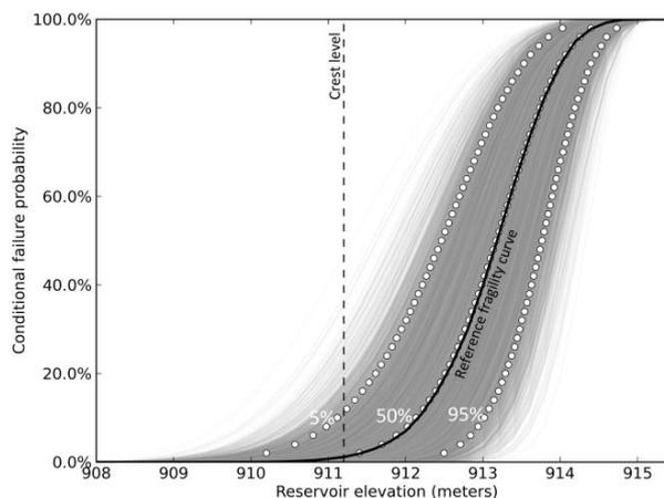
Figure 1: Family of fragility curves obtained for Dam A.
